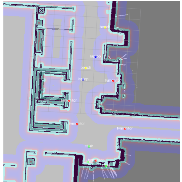
Figure 4: IGMM clusters visualized on the map using data from the object detection and localization pipeline.
