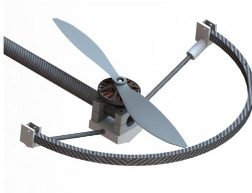
Figure 27: A rendering of a lower safety hoop surrounding one of the quadrotor propellers.
