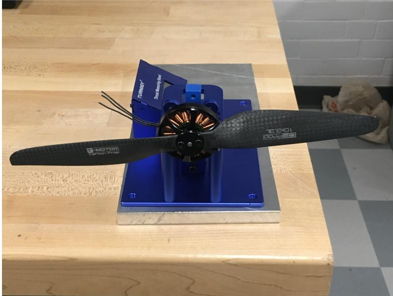
Figure 29: Antigravity 4004 motor and twisted blade on Turnigy thrust stand
