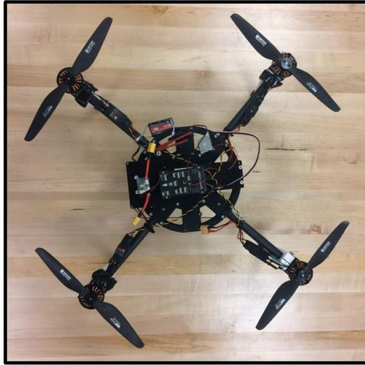
Figure 23: The quadrotor subsystem, assembled.
