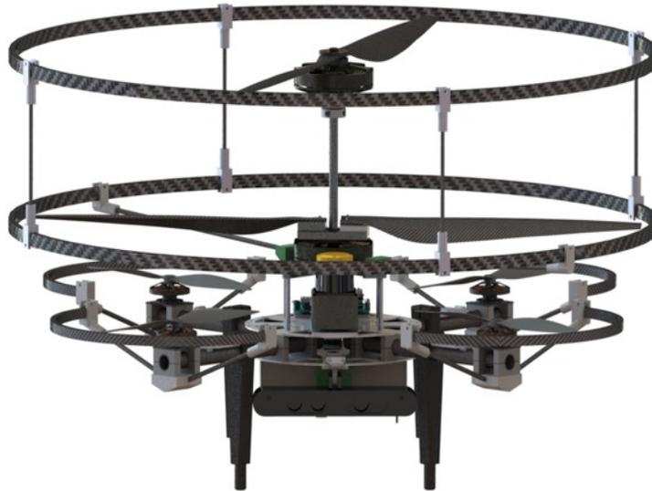
Figure 26: A Rendering of the OXcopter with the safety system
