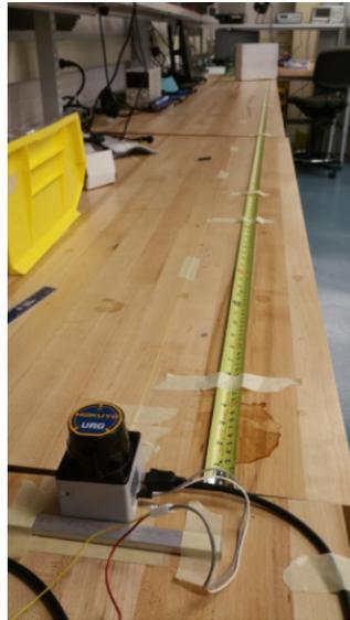
Figure 43: LiDAR testing setup
