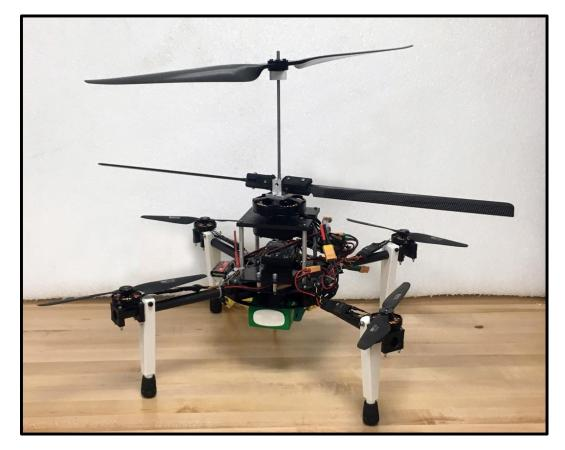
Figure 16: The initial design of the contra-rotating system, with a rotating shaft.
