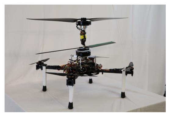
Figure 64: Final flight vehicle.
