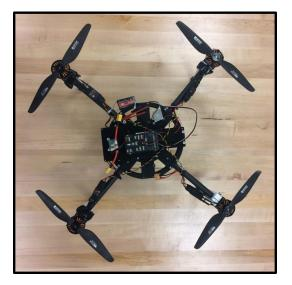
Figure 23: The quadrotor subsystem, assembled.
