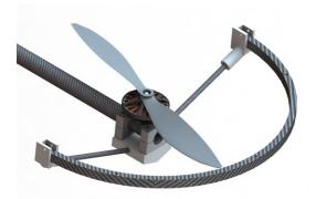
Figure 27: A rendering of a lower safety hoop surrounding one of the quadrotor propellers. The lower safety system consists of four, 10.9" outer diameter, 10.4" inner diameter semicir-
