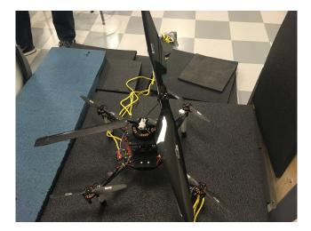
Figure 17: Bending failure of the first prototype.
