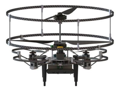
Figure 26: A Rendering of the OXcopter with the safety system
