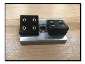
Figure 20: A photograph of angled wedges on the wedge adapter.
