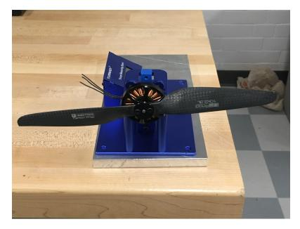
Figure 29: Antigravity 4004 motor and twisted blade on Turnigy thrust stand
